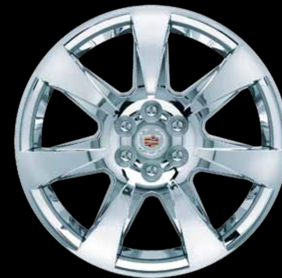
20" x 8" 7-SPOKE CHROME TECH CAST ALUMINUM WHEELS Available on SRX Performance and Premium Collections and includes P235/55R20 H-rated all-season tires
