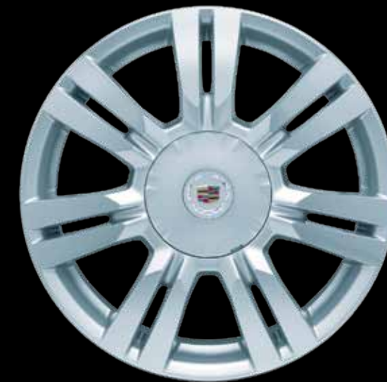
18" x 8" 7-SPOKE CAST ALUMINUM WHEELS WITH PAINTED FINISH Standard on SRX and includes P235/65R18 H-rated all-season tires
