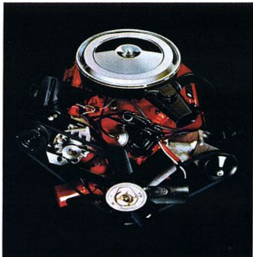
An entirely new engine for an entirely new automobile. The 350-4 V8. Standard equipment on the GS 350. 350 cubic inches. 4-barrel Quadrajel carburetor. Dual exhausts. Delivering 280 horsepower. 375 pounds feet of torque. The power you want. The dependable performance you want. And more economy than you'll believe.
