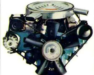
**SUPER WILDCAT**—Buick's mightiest V8! Twin four-barrel carburetors and a 425 cubic inch displacement give this magnificent engine a full 360 h.p. Optional on Riviera, Electra 225, and Wildcat. Use with Super Turbine (optional on Wildcat, regular equipment on Electra 225 and Riviera) or 4-speed transmission (optional on Wildcat).
