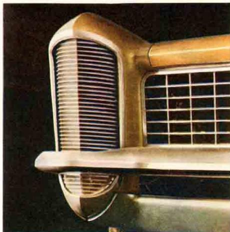
Something new in Riviera headlights. They're moved from the grille to a position behind the shields in the fenders. How do you open the shields? Simple, just pull the switch, they pop up out of the way. Push it in and the shields go down. Good way to amuse your friends.
