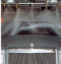
Body panel seals water-tested for leakage.
