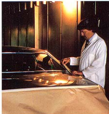
Body paint inspected for flaws.
