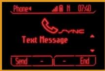
Operate the available SYNC voice-activated in-vehicle connectivity system with the 5-way control on the left spoke of the steering wheel, and the buttons on the center console. Follow the action on the 4-inch LCD display screen. Visit SyncMyRide.com for all the latest news.
