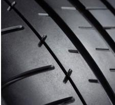
1. Do not use summer-only tires in winter conditions, as it would adversely affect vehicle safety, performance and durability. Use only GM-approved tire and wheel combinations. Unapproved combinations may change the vehicle's performance characteristics. Lower profile tires damage more easily; especially on rough roads. Damage is not covered under warranty. For important tire and wheel information, go to https://my.cadillac.com/learnAbout/cadillactires/ or see your dealer.
