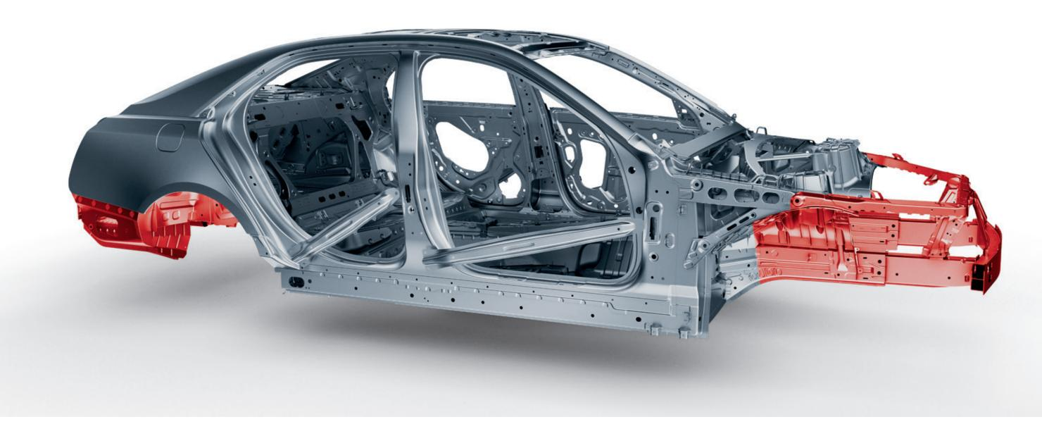
Constructed using ultra-high-strength steel, the CTS body incorporates crumple zones to help absorb and manage crash energy. And with 10 standard airbags,<sup>1</sup> including knee airbags for driver and front passenger and side-impact airbags for outboard rear passengers, CTS works to keep you protected at
