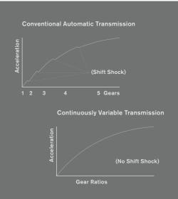
A smarter way to shift. The virtually "gearless" intelligent CVT (Continuously Variable Transmission) that makes shift shock and gear hunting a thing of the past. Fully variable gear ratios mean the CVT always delivers the right amount of power to the wheels whenever you push the throttle.
