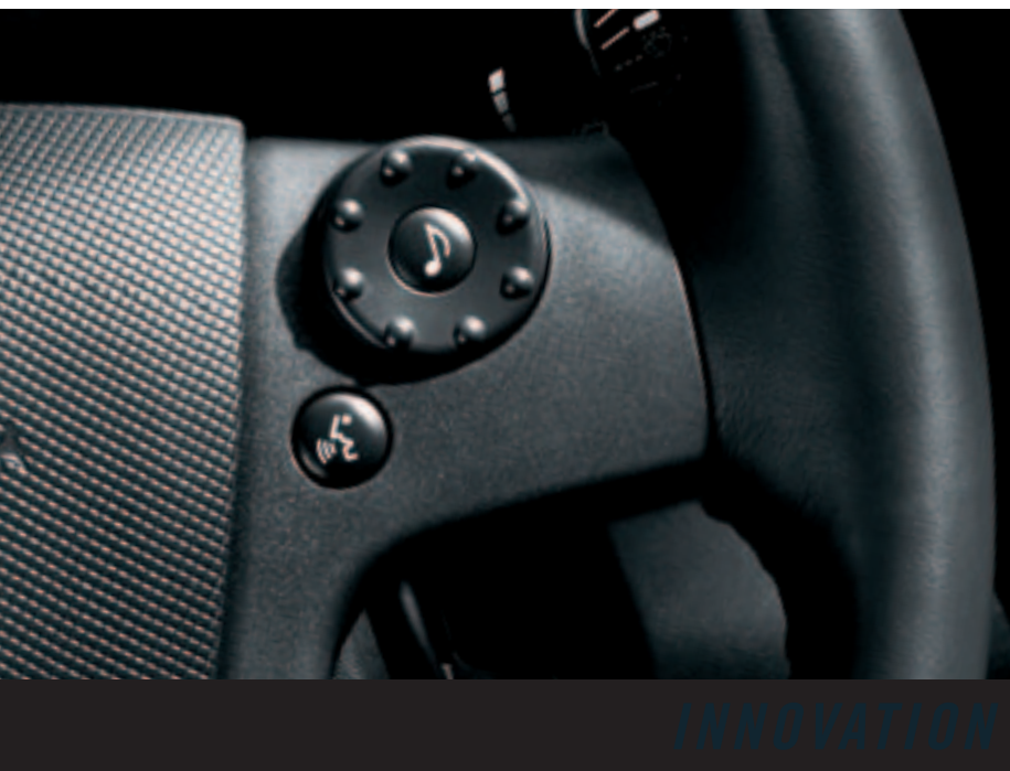
One of CTS's more innovative features is the steering wheel-mounted thumbwheel that lets you adjust the volume of the audio system and change the signal source without removing your hands from the wheel.
