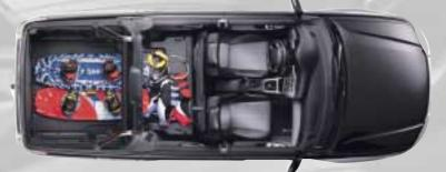
For maximum cargo space, you can drop the tailgate with the optional bed extender in place and lower the Switchback door for a cargo area over 90 inches long
