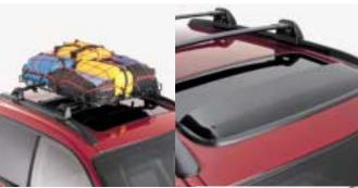
Hood protector. Durable acrylic plastic wrap-around design helps protect the Baja hood from stone chips and bugs.
