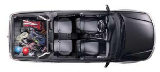
With the Switchback door closed, you have plenty of room for four and a cargo bed floor 41.5 inches long by 49 inches wide.
