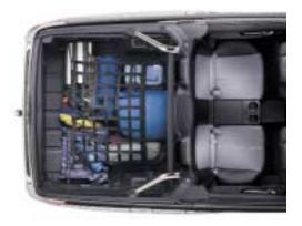
To help secure your gear, the cargo bed features four tie-down hooks that can be used with with the optional bed cargo net.
