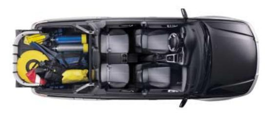
For maximum cargo space, you can drop the tailgate with the optional bed extender in place and lower the Switchback door for a cargo area over 90 inches long. Or with the Switchback system closed (as shown), and you have a cargo bed over 58 inches long and still have seating for four.
