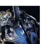
Baja is powered by a 2.5-liter, 16-valve horizontally opposed boxer engine producing 165 horsepower and 166 lb.-ft. of low-end torque.
