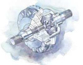
Baja models feature a standard limited-slip rear differential that further enhances traction. If one rear wheel starts to lose traction, power is automatically diverted to the other rear wheel-all without the need for driver intervention.
