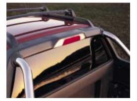
Looking for something? The standard dual illuminated cargo bed light makes nighttime loading and unloading easier.
