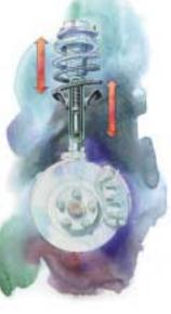
As the body of a vehicle leans in a turn, the suspension of the inside wheels extends. All Baja models feature a rebound spring inside the front strut that is designed to use the mass of the wheels, tires and brakes to resist this extension, reducing body roll in turns. The rebound spring also works to reduce the lift of the nose of the vehicle during acceleration.
