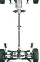
Powertrain components are laid out in a straight line and close to the chassis' centerline, giving agility while providing greater stability.
