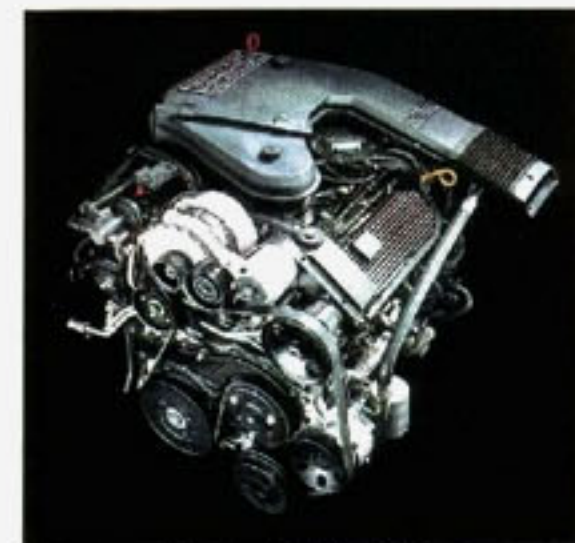
Transverse-Mounted 4.1 Liter V8 Engine.
