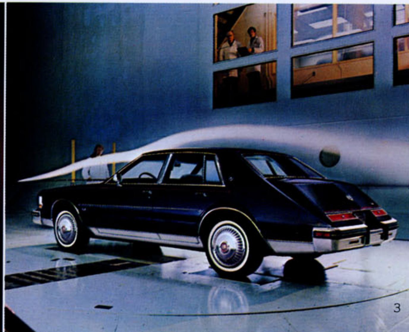
Wind Tunnel testing for aerodynamic efficiency.
