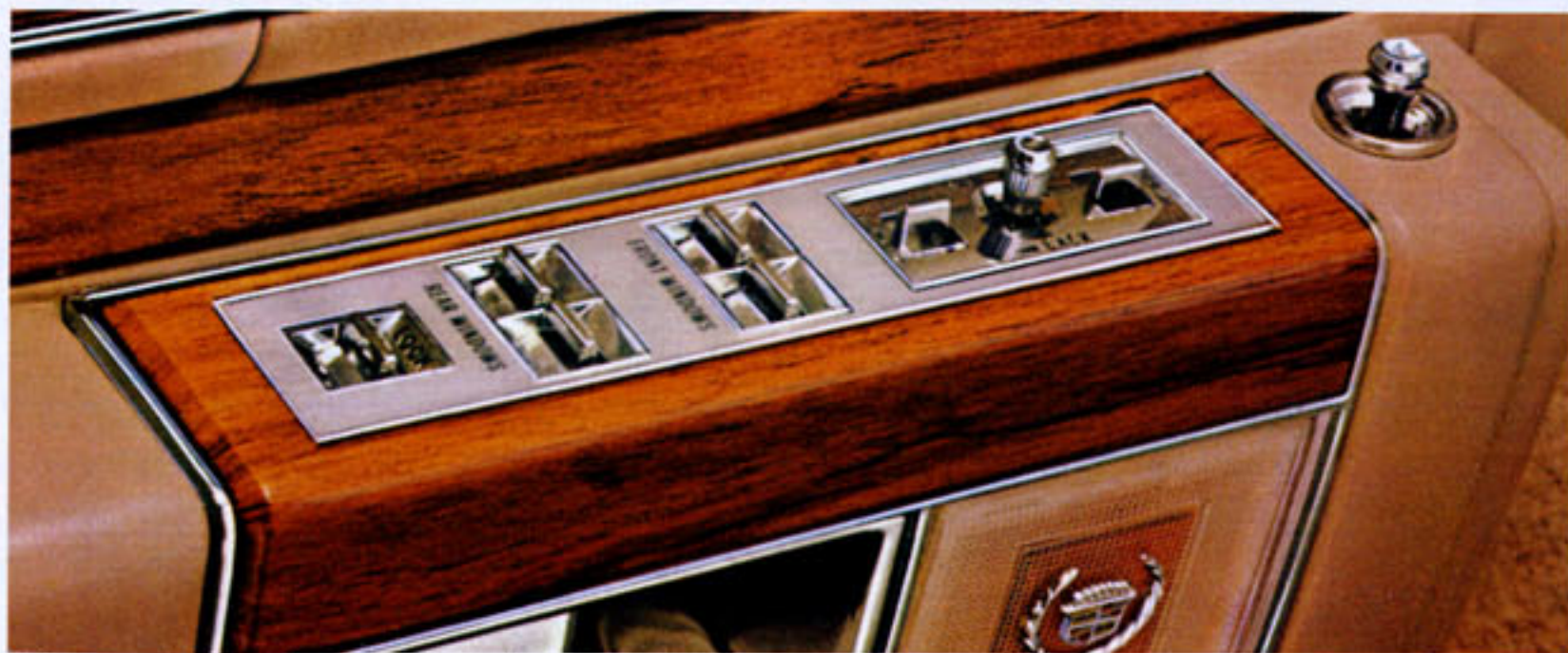
Power control panel on the driver's door armrest.
