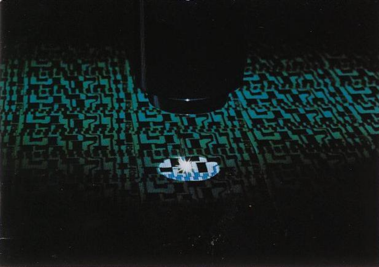
Laser trimming of Electronic Control Unit for Cadillac's exclusive Electronic-Fuel-Injected Engines.
