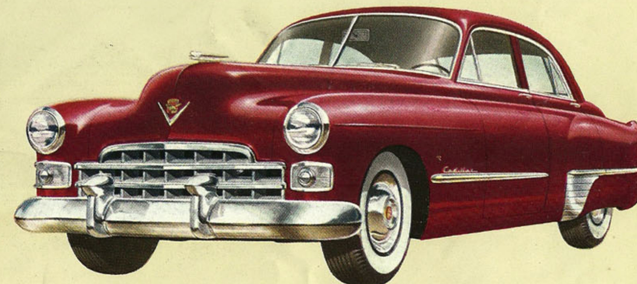
A greatly increased effect of lowness and breadth has been achieved in the new Cadillac front-end design for 1948. New features include the graceful forward slope of the hood, the heavier and more massive bumper, and the lower grille.
