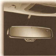
The Electrochromic inside mirror on Series II automatically dims to reduce glare by up to 94 percent.
