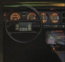
ABOVE: The GTA's duplicate radio controls on the steering wheel hub made it easy for the tunes to just keep on comin'.
