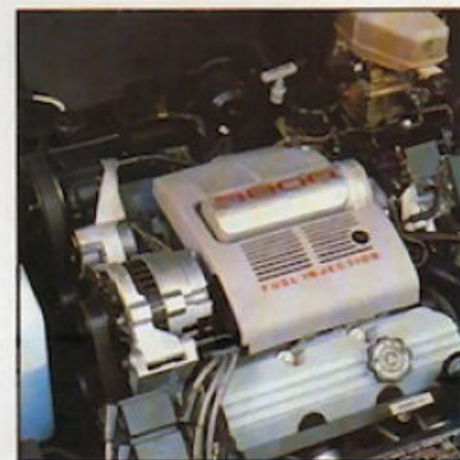
LEFT & FAR LEFT: Bonneville SE comes standard with a new 3.8 liter SFI 3800 V6 engine that features sequential port fuel injection and 165 hp. It's the same standard powerplant found in the SSE, left center.
