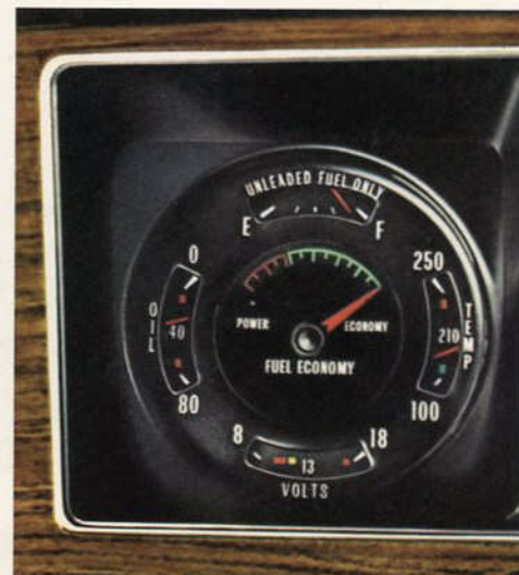
Available Fuel Economy Gauge. It lets you know when you could be getting better gas mileage.
