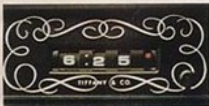
Oldsmobile's new digital clock gets special treatment in the Regency—its facing is styled and signed by Tiffany & Co. The movement is quartz-crystal controlled for exceptional accuracy.
