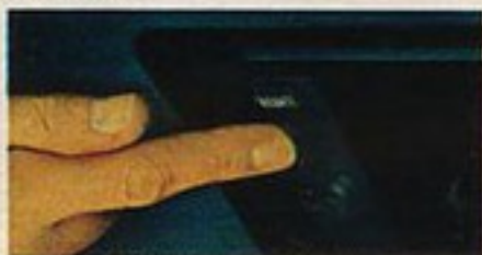
Just touch this button, and you've released the tailgate from the driver's seat. It's interlocked with the ignition—so you can't release it accidentally while in motion.
