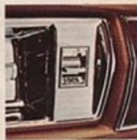
Power door locks secure all doors with a switch in the driver's door.
