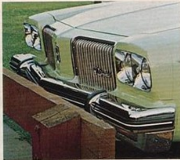
Front and rear bumpers are mounted on hydraulic cylinders which cushion minor impacts.
