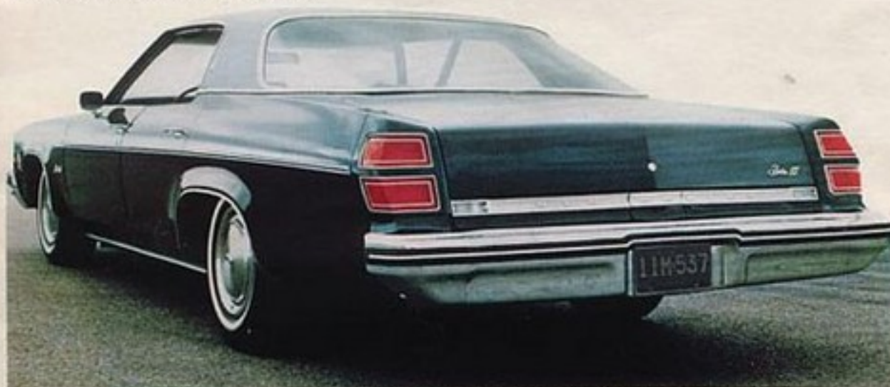
With taillamps stacked vertically in the fenders, Delta 88's trunk opening comes down close to the bumper across its full width—requires less lifting than some other cars to clear the sill.
