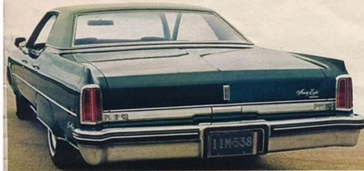
A new hydraulic rear bumper system is now standard, as are bumper impact strips and bumper guards. Note the exceptionally low trunk sill, for easy packing and unpacking.
