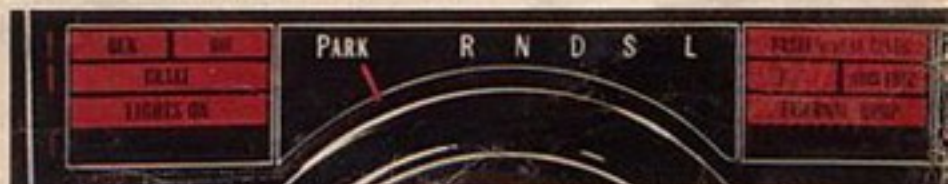
Oldsmobile's message center is arranged in two panels flanking the Hydra-matic quadrant, signals you when any one of many functions requires your attention.
