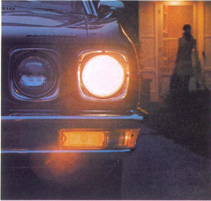
Headlamp Delay (Code 672—UPC T81). New and available all models. Allows you to have lighted path to house by turning off headlight switch after ignition is turned off. Headlights automatically stay on for 60 seconds and then go off. (F,D)
