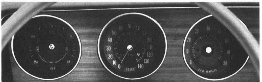
Rally Gauges with Clock (Code 488—UPC W63). Integrates oil, water and fuel gauges with alternator telltale on Tempest, LeMans, LeMans Sport, GTO and Grand Prix. Also includes clock, where not already standard. Rally Gauges with Instrument Panel Tachometer (Code 484—UPC U30). Same as above, but with tachometer substituted for clock. Illustrated on LeMans model. (F)
