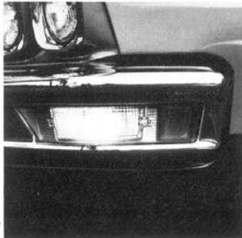
Cornering Lamps (Code 651—UPC T87). Available Catalina, Executive, Bonneville and Grand Prix only. Part of Lamp Group (Code 322). Light up blind spots when turning. Operate when headlights are on and turn signal is activated. Mounted on forward side of front fender and integrated with parking side marker lamp. (F)
