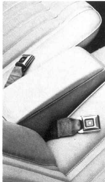
Custom Seat Belts and Front Shoulder Belts (Code 451—UPC AK1). Features compact, press-to-release pushbutton buckle on fixed-length belt for driver and outboard passenger. Front outboard belt adjustment is made automatically after belt hookup by outboard retractor which takes up slack and provides desired tension. All other belts adjust in the conventional manner. All belts, front and rear, available in seven harmonizing colors. Available all models. Also available are Custom Seat Belts and Front and Rear Shoulder Belts (Code 452—UPC AK2). (F)
