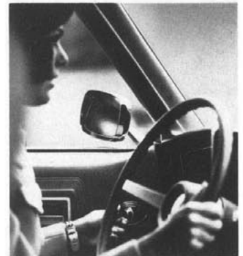
Remote-control Outside LH Mirror (Code 444—UPC D33). Mounts on door. Adjusted by convenient controls inside car. Available all models. (F,D)
