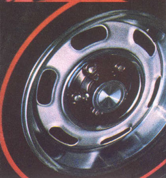
A very sporting extra-cost combination. Redline wide oval tires and polished steel Rally I wheels. The wheels are available only with disc brakes. (The wide ovals are standard on all Firebirds.)
