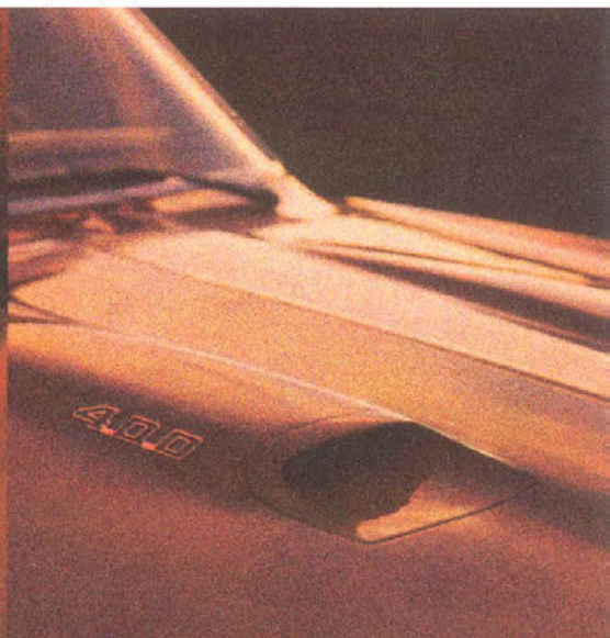
Those scoops are real with the 400's Ram Air option. This induction system, combined with a different cam and valve springs, lifts the hp peak above 5000 rpm. Extra-cost, but you get what you pay for.
