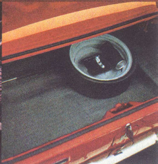
The Space Saver Spare. Adds 3 cubic feet of usable space to the luggage compartment. Deflated, but if you ever need it, a pressure can, packed with the tire, inflates it in seconds.
