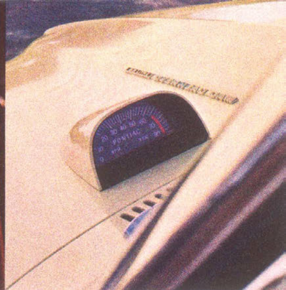
The hood-mounted tach lets you shift properly without looking down from the road. (You do use a tach for shifting, don't you?)
