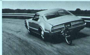
Fifth-wheel records every move test car makes!
