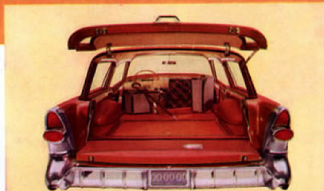
The New Buick Estate Wagons Are As Big In Roominess As They Are Low In Profile. Rear seats fold down to provide a 701.9-inch-long platform from front seat to end of open tailgate. Maximum width of the opening is 61.2 inches. Maximum height is 27.6 inches. Two accessories make this versatile Buick even handier—a divided rear seat for carrying both passengers and cargo—and a third seat for children which gives your Estate Wagon 9-passenger capacity.
