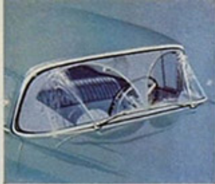
Automatic Windshield Washer —plays two adjustable jets of water on windshield, while wipers clear away dirt. Shuts off automatically. Standard on ROADMASTER, optional on other Series.
