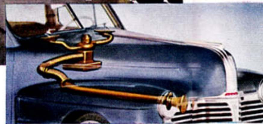
THE DEFROSTER illustrated, furnished with Underseat Heater, provides a large volume of hot or fresh air which may be tempered to suit the passengers.
