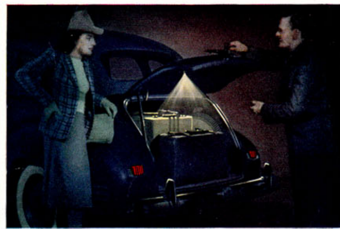
A LUGGAGE COMPARTMENT LIGHT is available for installation on the inside of the compartment door. This light turns on automatically when the door is opened and illuminates the entire compartment. A great convenience in removing luggage or spare tire at night.
