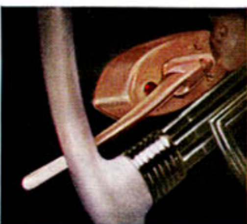
DIRECTIONAL SIGNALS enable you to indicate a right or left turn to cars coming from either front or rear by moving a lever forward or backward.
