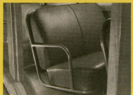
CENTER SEAT ARM REST. A convenient metal arm rest on the center seat provides support for the right hand passenger while rounding curves and turns.
