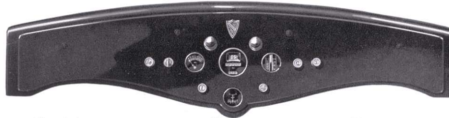
Speedometer . . . ammeter . . . oil pressure gauge . . . gasoline gauge . . . choke and throttle control . . . combined light switch and semi-coincidental transmission and ignition lock . . . each individually mounted on a new ebony finish instrument board
