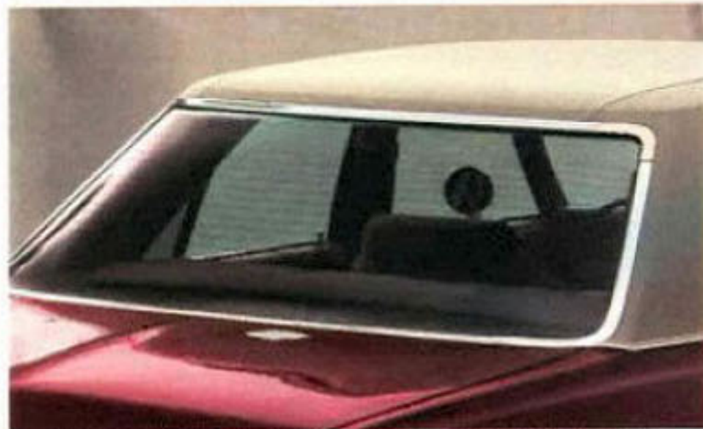
Electric Rear Window Defroster, with heating elements bonded to the glass, quickly clears window of frost, snow and ice.
