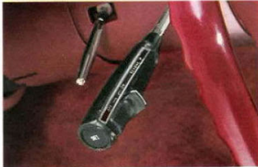
Automatic Speed Control lets you select and hold a steady speed for ease in highway driving.
