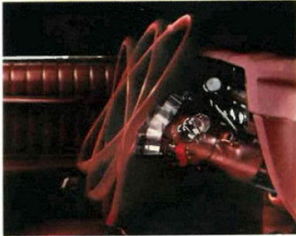
Tilt Steering Wheel, shown here in three of its seven positions, adjusts up and down for easy entry and exit.
