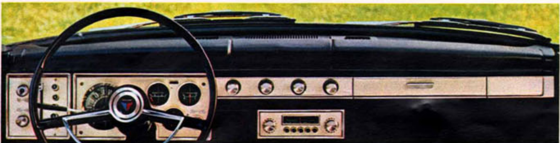
Signet dash panel gauges show speed, fuel, alternator and engine temperature at a glance. Ash receiver, glove box and lighter, all are within convenient reach.
