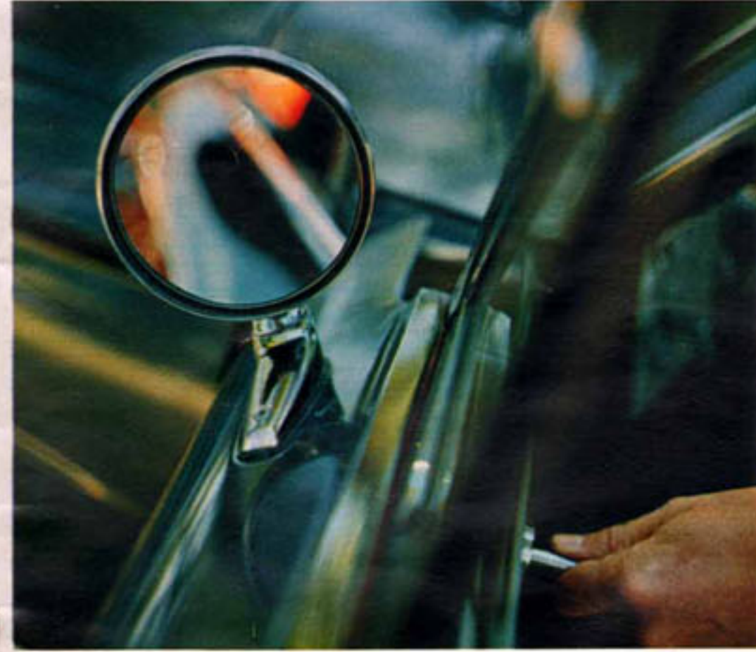
Remote control outside mirror with control lever located on inside door panel, driver can conveniently adjust mirror for best vision.
