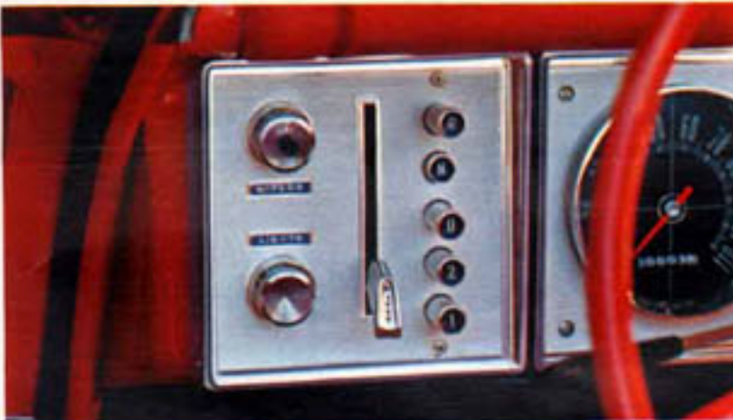
Automatic 3-speed TorqueFlite transmission shifts for you at precisely the proper engine speeds. Automotive engineers call this the finest in the industry.
