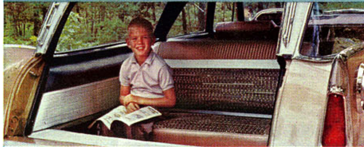
REAR-FACING THIRD SEAT, another "first" for Plymouth, permits generous legroom and hiproom for adults, and has proved very popular with children. (Unlike third seats on some wagons, it folds into floor.)
