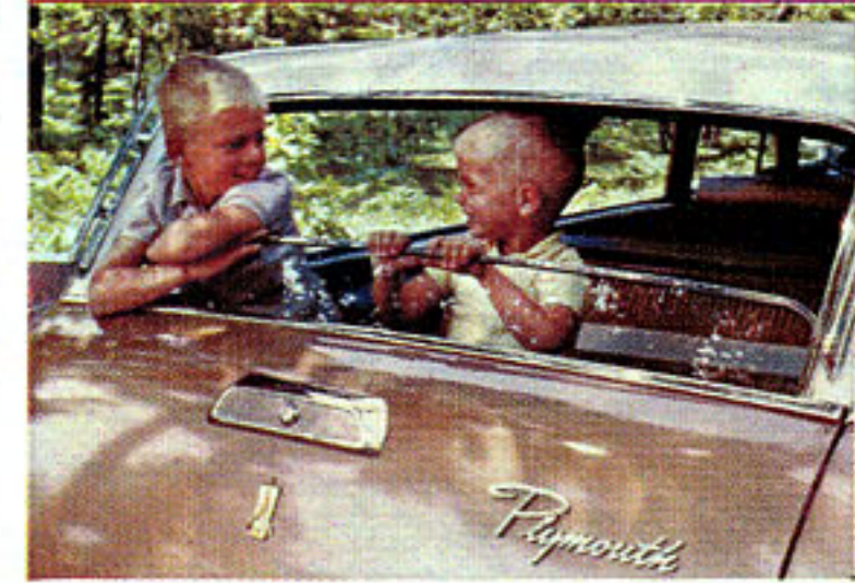
ROLL-DOWN REAR WINDOW was introduced to its field by Plymouth and is found on every Plymouth wagon. Electric control (by handy driver button or by key outside tailgate) standard on Sport models, optional at quite low extra cost on the other two series.
