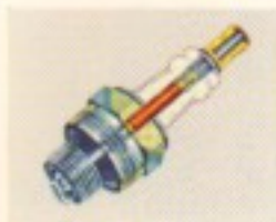
Longer-life resistor spark plug has extra-wide gap which gives smoother engine idling and saves on fuel.
