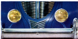
FOG LAMPS . . . Provide Protection and convenience for driving in adverse weather. Mount low on bumper bracket easting.
