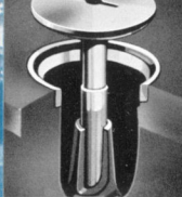
Exhaust Valve Seat Inserts. Are of heat-resisting alloy steel. Valves seldom need attention under 30,000 miles.
