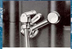
Manifold Heat Control. During the warming-up period, this automatic control aids in vaporizing gas mixture before it enters cylinders.
