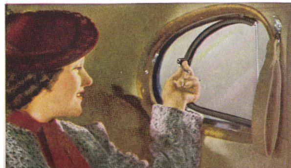
Draught Free Ventilation in both front and rear compartments controls the amount of fresh air that is permitted to circulate within the car's interior.
