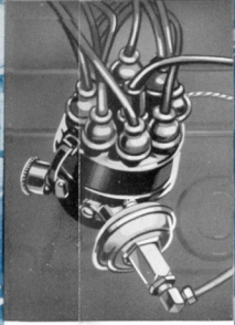
Vacuum Spark Control. Automatically advances or retards the ignition spark to the point of maximum efficiency and economy.
