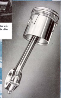
Aluminum Alloy Pistons. Light weight, astonishingly long-wearing. Four rings provide effective oil and compression seal.
