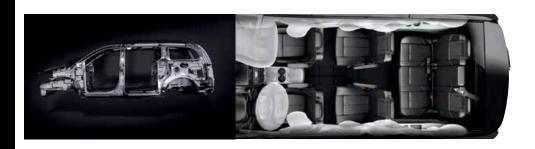
STRATEGICALLY PLACED HIGH-STRENGTH STEEL. Town & Country architecture includes dual-phase, high-strength and hot-stamped steel, resulting in a strong safety cage that contributes to overall vehicle-impact performance.
