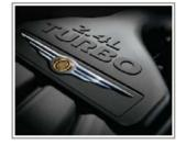
PT Cruiser Convertible's standard 2.4-liter DOHC 16-valve 4-cylinder power plant offers 150 horsepower at 5,100 rpm and 165 lb-ft of torque at 4,000 rpm. You'll appreciate those numbers when you step on the gas pedal to climb a hill or pass another vehicle.
