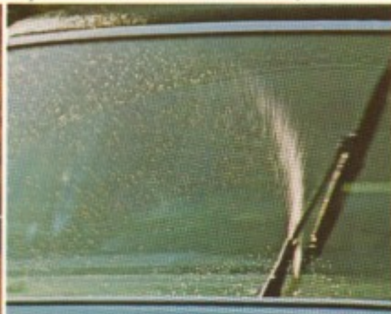
Wiper mounted windshield washer jets
