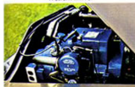
Heavy-duty cooling units provide optimum reliability. Optional 110/120-volt, 2500-watt Electric Power Pak is a self-contained unit.
