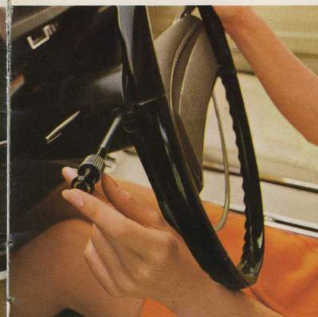
Automatic speed control, at tip of turn signal
