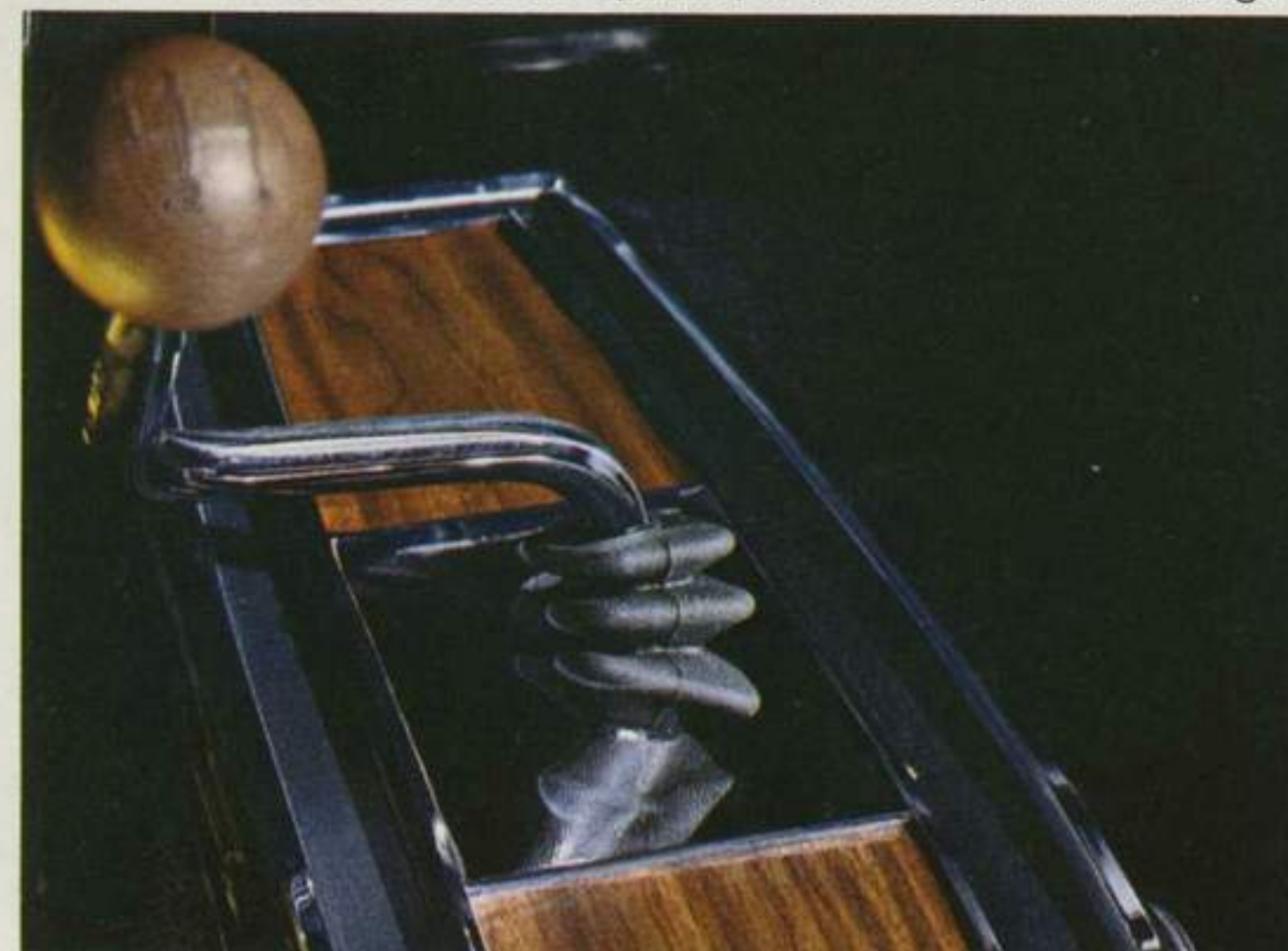
Charger R/T's four-on-the-floor, with Hurst linkage
