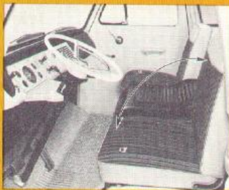
A. Battery Accessibility
