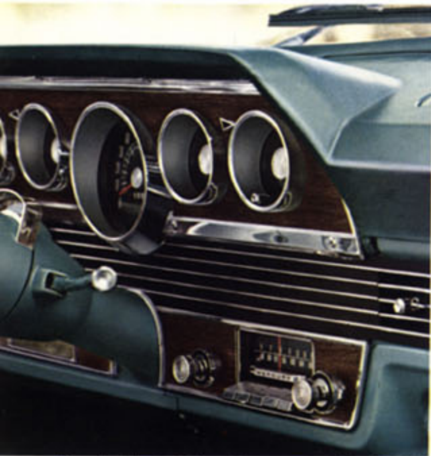
More dash in the Caliente instrument panel for '66. Simulated wood-grain finish outlines the big-dial speedometer and other conveniently located, easy-to-read instruments.
