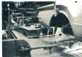
Bodies are actually immersed seven times for special cleaning, rinsing, and rustproofing treatments after welding.
