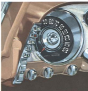
THE PUSH-BUTTON Drive Selector panel is conveniently located to the left of the steering wheel, out of everyone's reach except the driver. The five buttons are illuminated for night driving.
