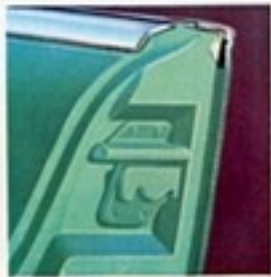
New Safety Lock door latch—a unique safety feature designed to keep doors safely closed under sudden impacts...now standard equipment on all 1956 De Soto models.
