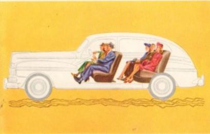
The new Mercury has mid-section seating. Rear seat passengers are located well ahead of the rear axle center line where the least amount of car movement occurs when negotiating rough roads. The result: a smoother, more level ride. Balanced weight distribution in combination with new slow-motion multileaf springs and a 129.38 inch spring base results in a full-cushioned ride.
