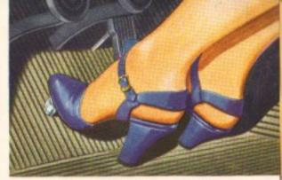
Safety foot control permits instant tuning without removing hands from whoel... a convenience as well as a safety feature. Partially depressing foot control serves as temporary silencer, for easy conversation.
