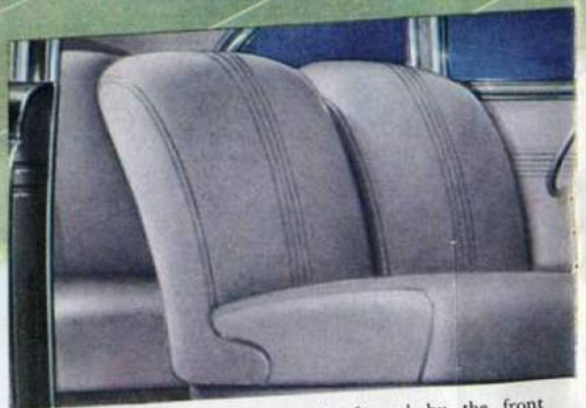
A CONTINUOUS CUSHION support is formed by the front seat backs. The wide rear seat is easily accessible because front seat back is divided, and either side tilts forward and inward.
