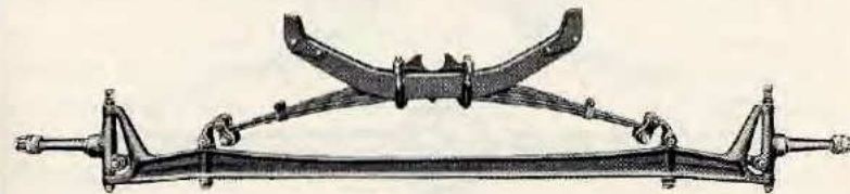
Front axles on all Model T Cars are each drop-forged from one single ingot of Vanadium steel especially heat-treated in our own plant
