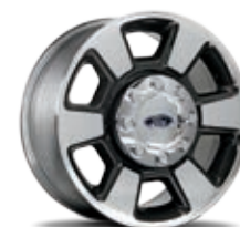
18" Bright-Machined Cast-Aluminum Standard: F-350 SRW
