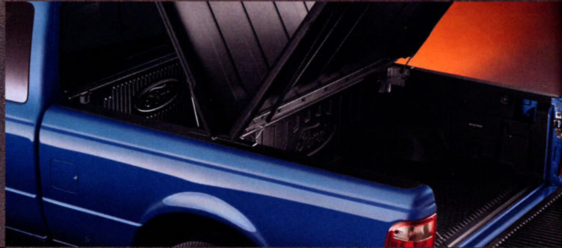
Optional Lockable Two-Way Hard Tonneau Cover keeps things dry as well as out of sight. Also available with divider panel that acts as a compartment organizer.
